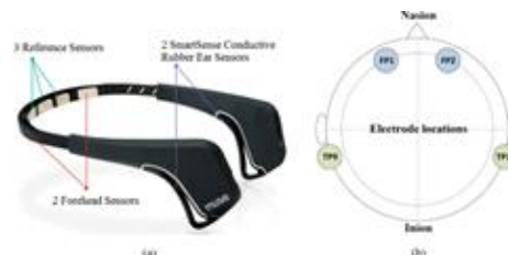
Figure 1. Muse EEG recording device and its electrode positions (Liu et al., 2020)
